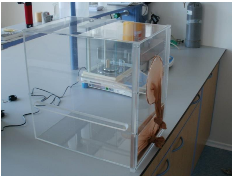
Figure 1 Experimental transparent acrylic cage, measuring approximately 40 cm x 40 cm x 25 cm (40,000 cm 3 ), with a sleeved fabric opening for access from the front
